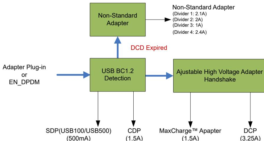
**Figure 2-1. DPDM Detection Process**
