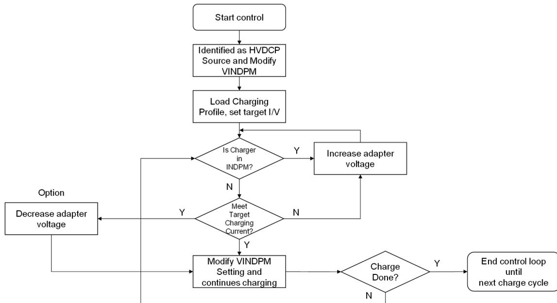
Figure 2-6. HVDCP/PPS Fast Charging Flow Chart
