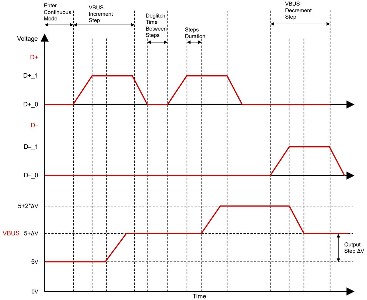
**Figure 2-7. Adjustable Adapter Output Step by DPDM Interface**
