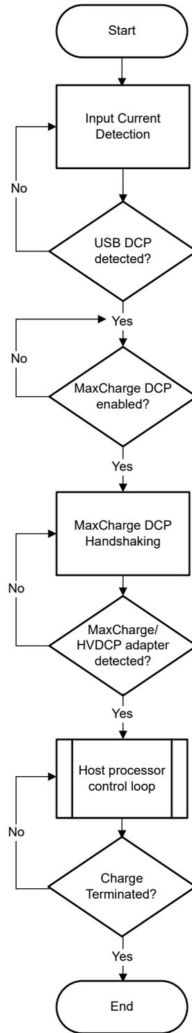
Figure 2-2. DPDM Working Flow Chart
