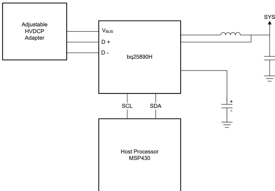
**Figure 2-5. Simplified Schematic of BQ25890H for PPS/HVDCP Power Source**
