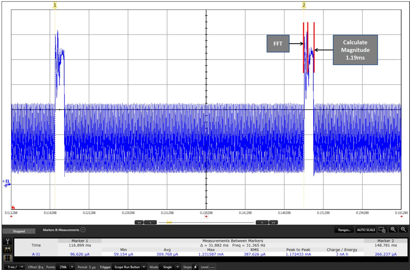
图 14. FFT With LEA Without BoosterPacks Average Current Consumption
