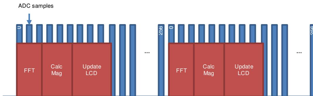
图 3. Generic Timing Diagram for FFT Operation
