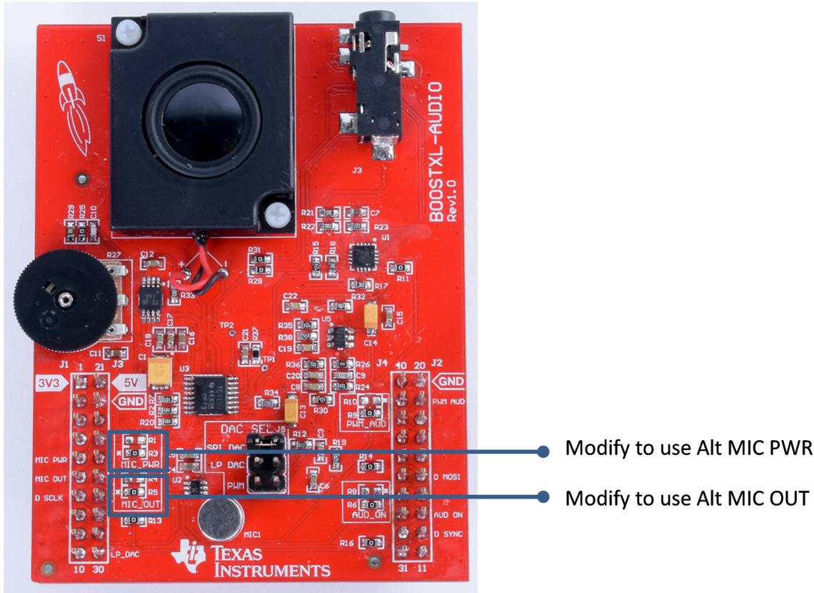
图 7. BOOSTXL-AUDIO BoosterPack Required Modification
