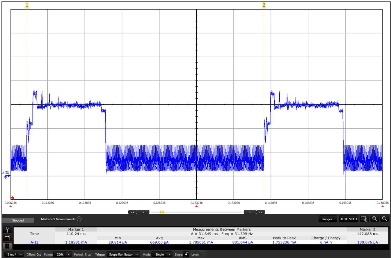
图 15. FFT Without LEA Without BoosterPacks Current Consumption
