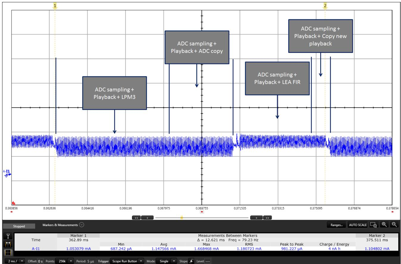
图 17. FIR Average Current Without Audio BoosterPack and Graphics LCD
