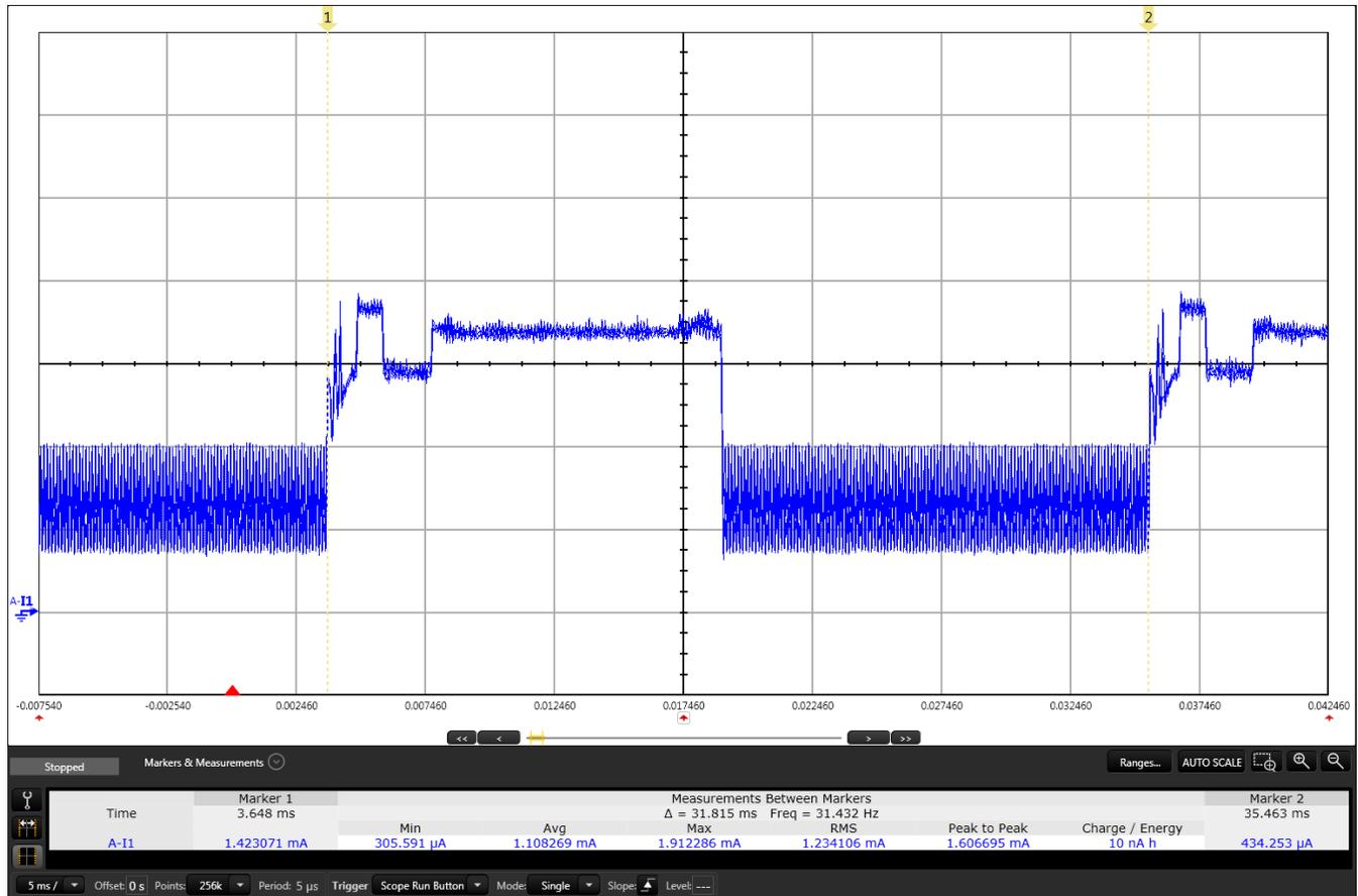
图 13. FFT With LEA, Audio BoosterPack and Graphics LCD Average Current Consumption
