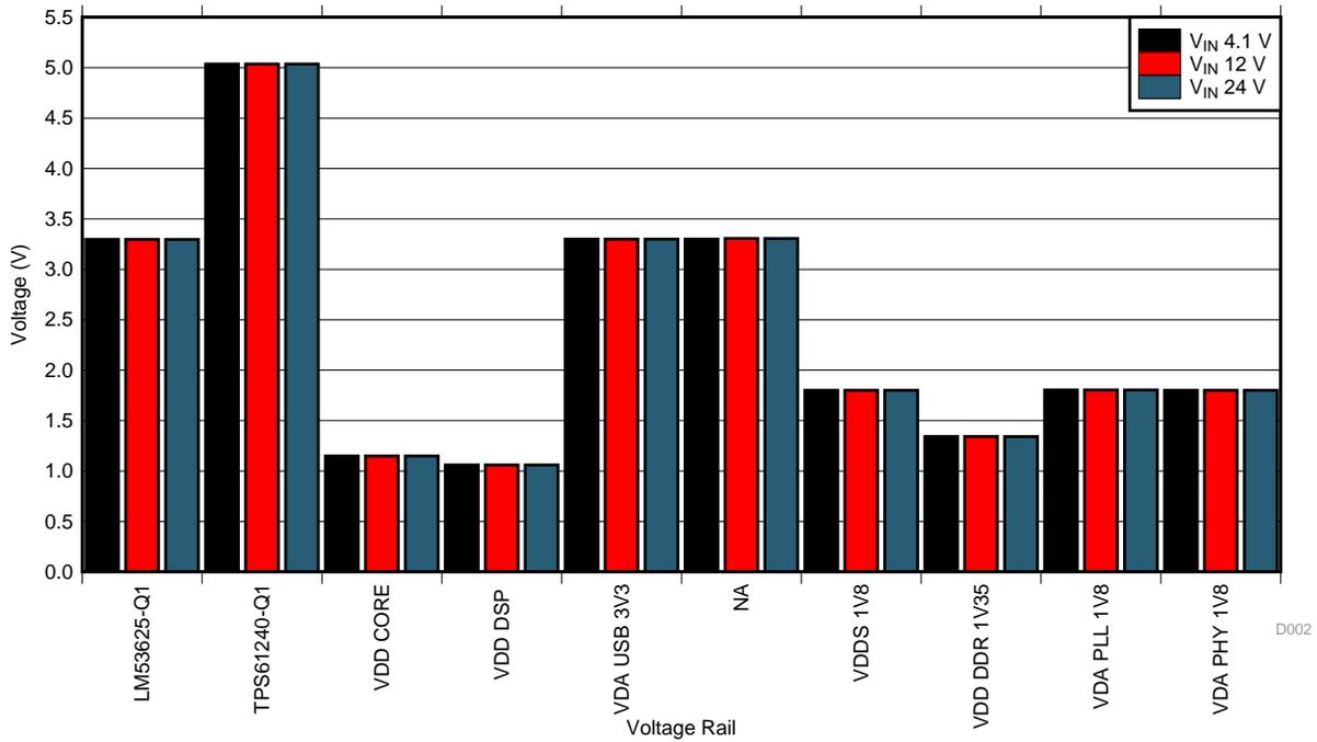
图 38. TIDA-01425 Voltage Rails versus Input Voltage
