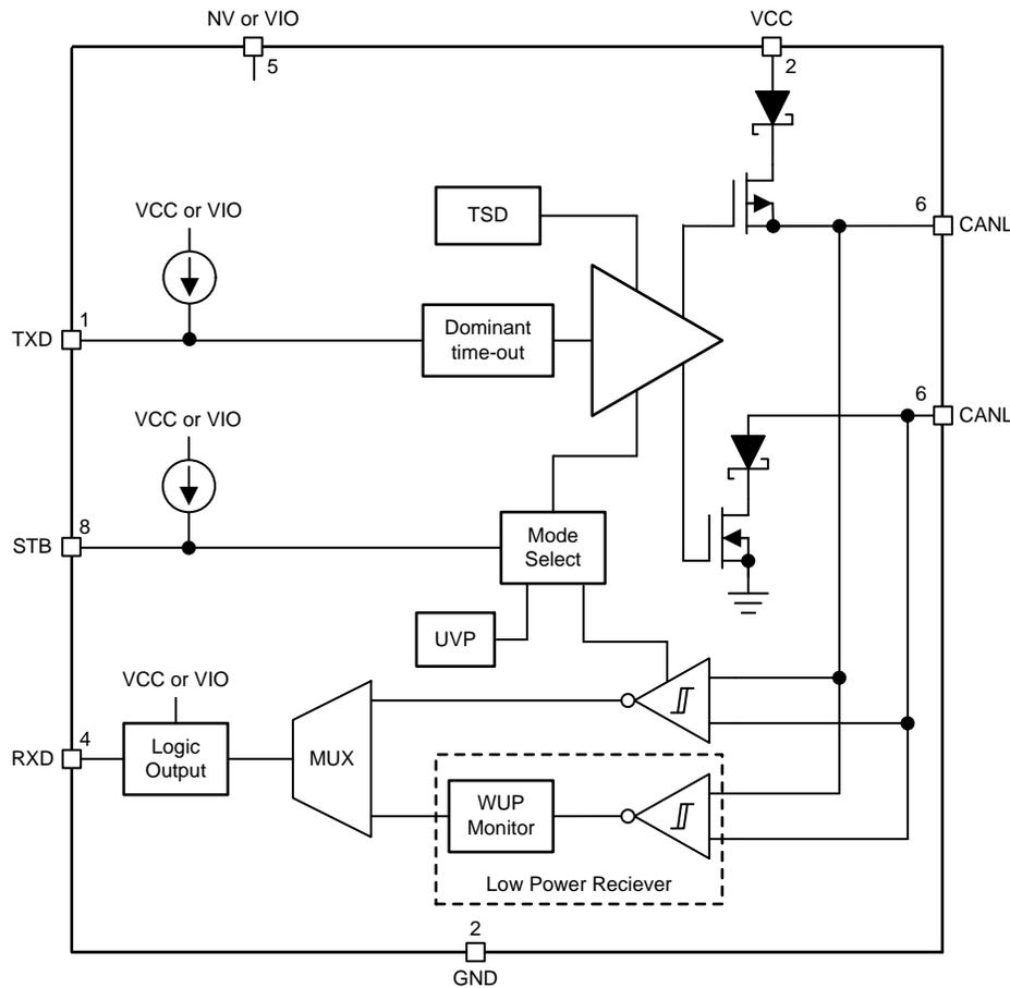
图 5. TCAN1042-Q1 Functional Block Diagram
