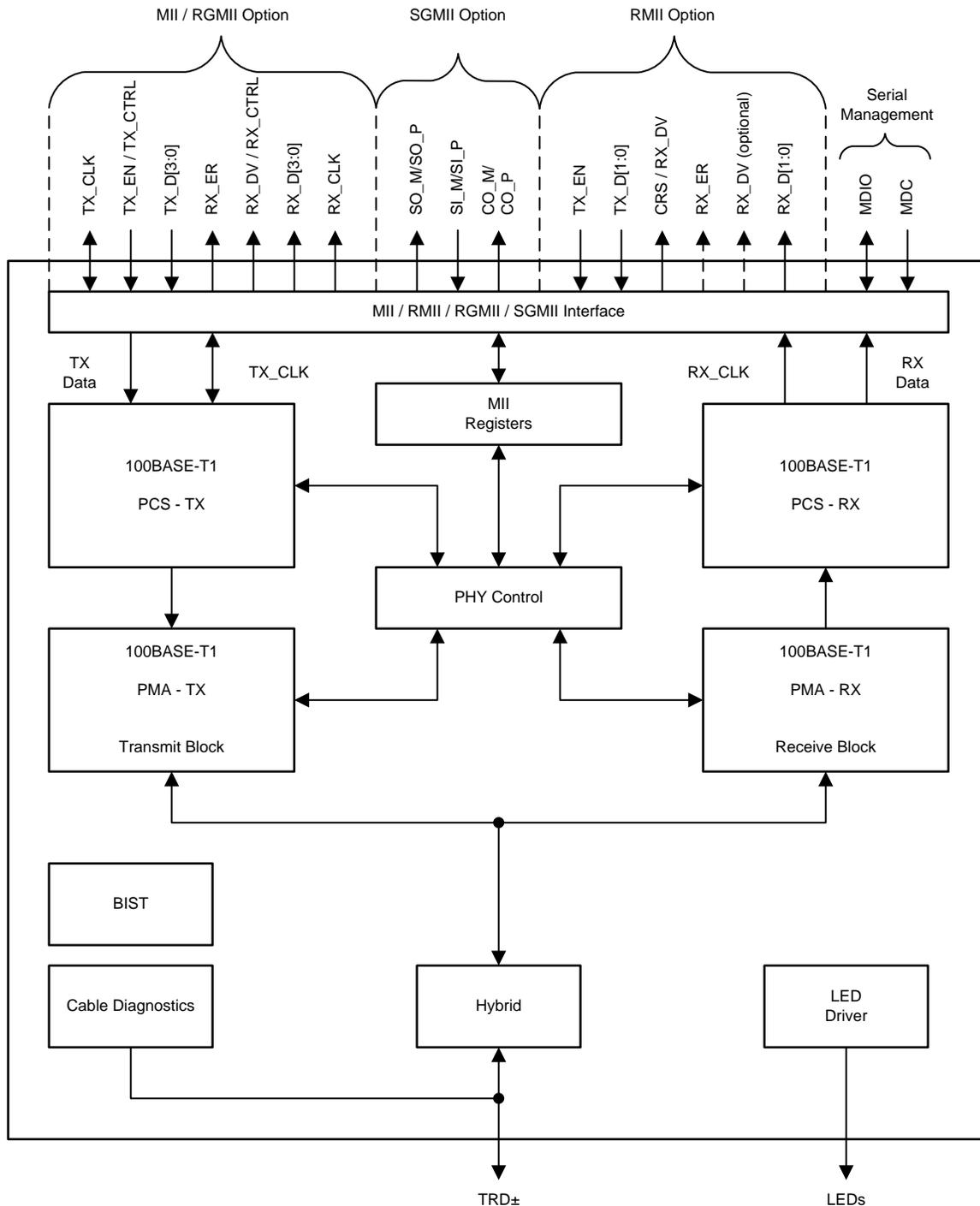
图 3. DP83TC811RH-Q1 Functional Block Diagram
