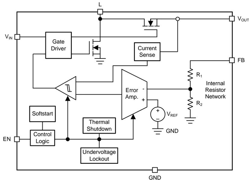
图 10. TPS61240-Q1 Functional Block Diagram
