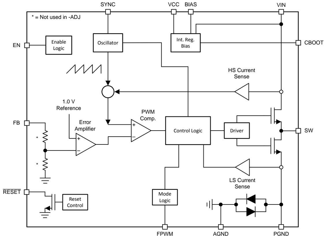
图 7. LM53625-Q1 Functional Block Diagram
