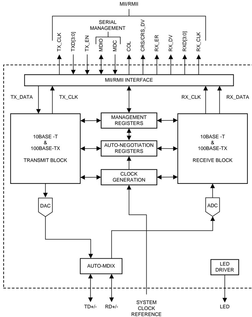
图 4. DP83848Q-1 Functional Block Diagram
