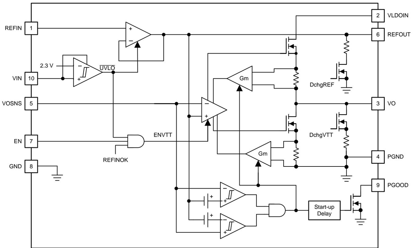
图 11. TPS51200-Q1 Functional Block Diagram
