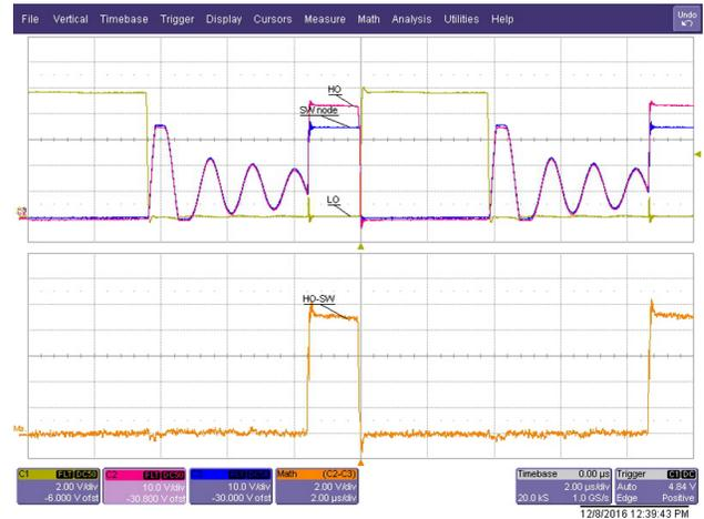
图 68. Switching Waveforms With Fixed Dead-Time Settings (R906 = 10 k)
