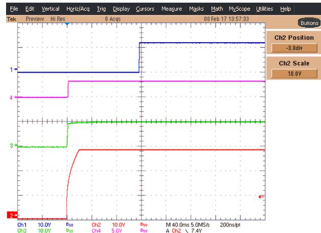
图 89. Start-Up Behavior of All Bias Power Supplies—Start Initiated by EN12 From 12-V Battery Terminal: (Blue = P12V, Violet = P3V3, Green = P10V, and Red = VIN\_LM)
