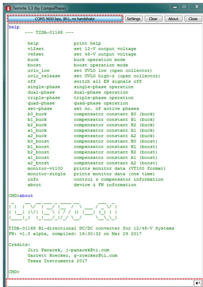
图 61. Interfacing TIDA-01168 With Serial Terminal Using Termit 3.3
