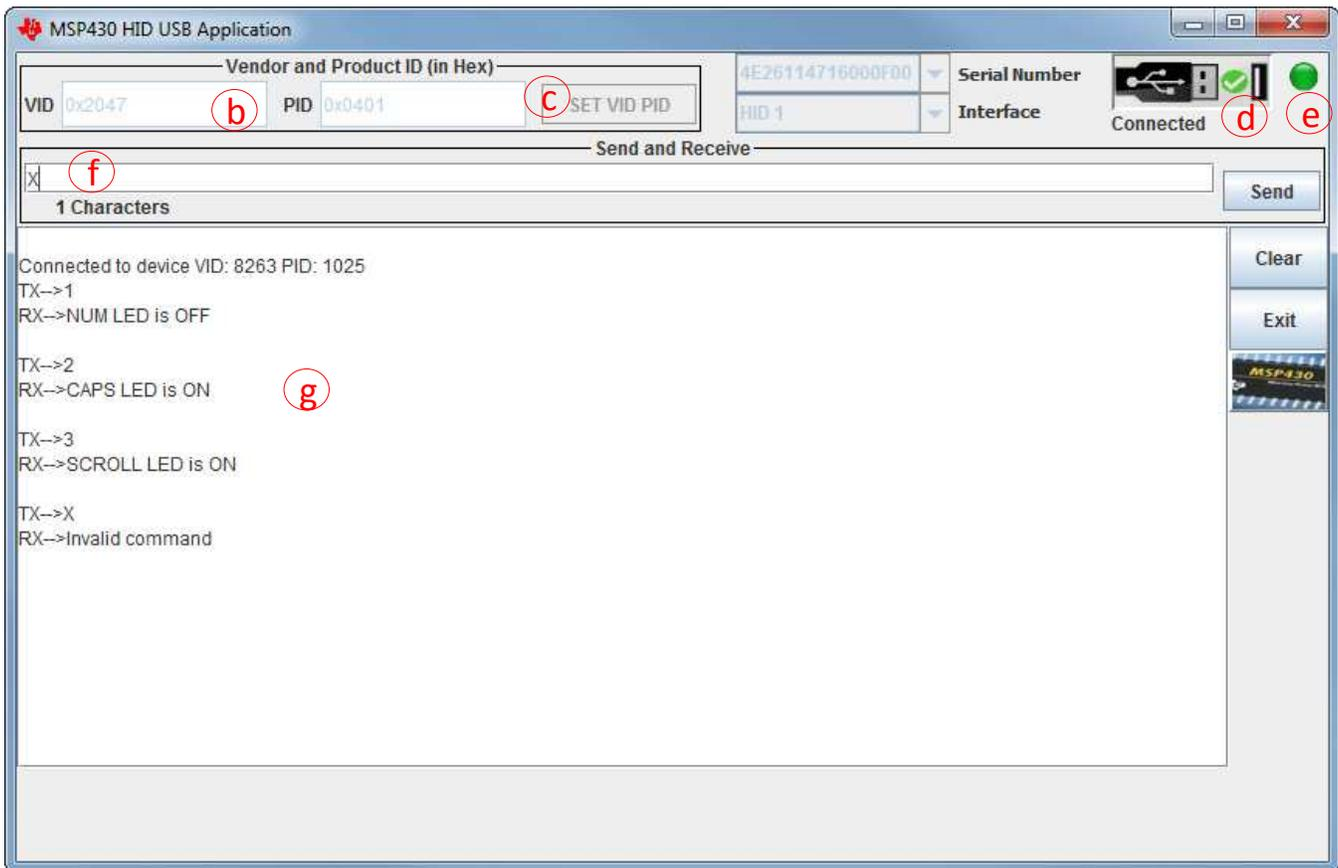
**Figure 20. Testing the HID Custom Interface using MSP430 HID Demo**
