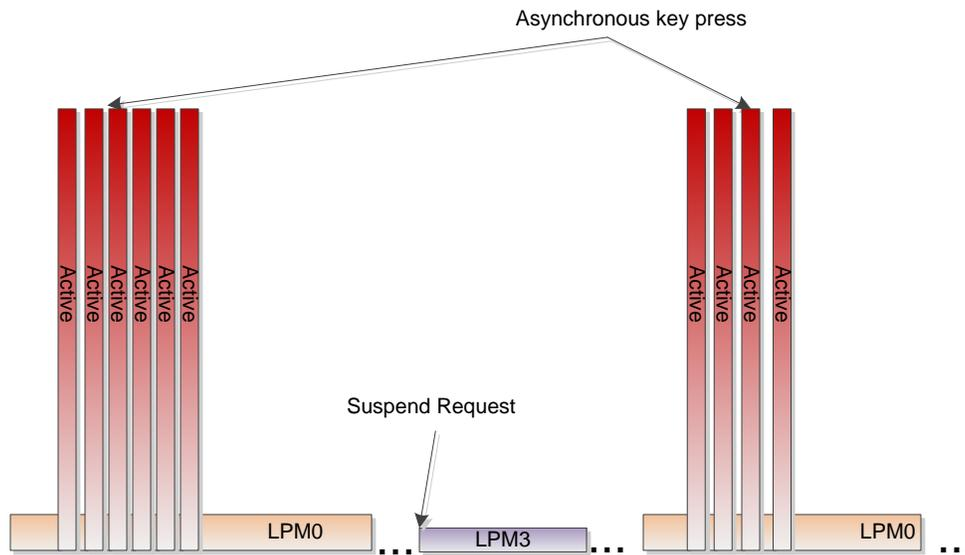
**Figure 29. Expected Power Profile for USBKBD Configuration**
