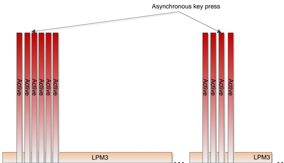
Figure 27. Expected Power Profile for *I2CKBD* and *I2CKBD\_G2xx4* Configurations
