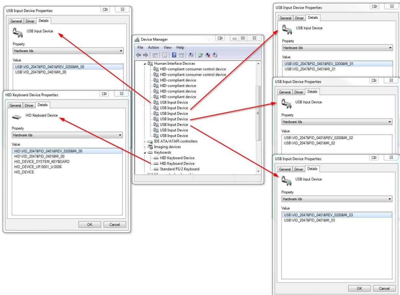
**Figure 19. USB Keyboard in Windows Device Manager**
