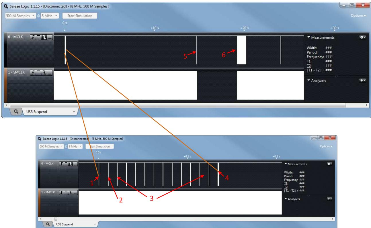
**Figure 30. Power Profile Observed on USBKBD**
