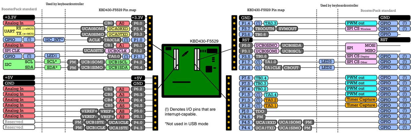
Figure 15. Pinout for Boosterpack Connector using MSP430F5529
