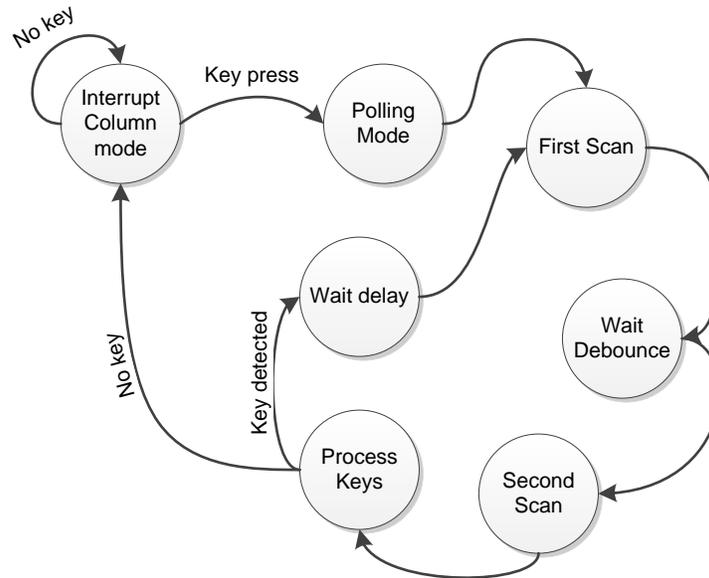
**Figure 14. State Diagram for Keyboard Scan**
