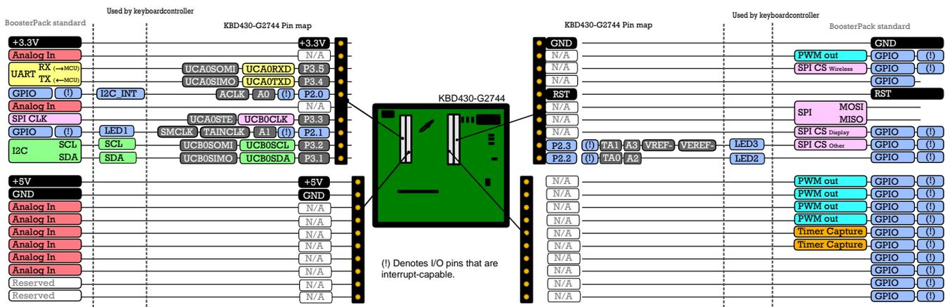
Figure 16. Pinout for Boosterpack Connector using MSP430G2744
