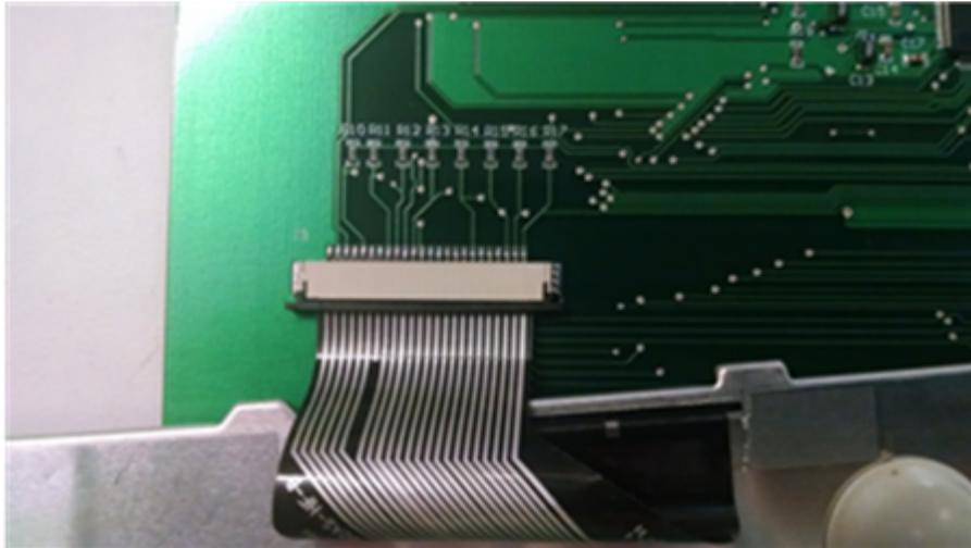
**Figure 18. Keyboard Connection**
