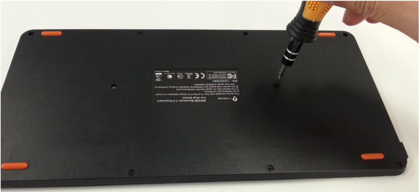
**Figure 4. Remove Screws**
