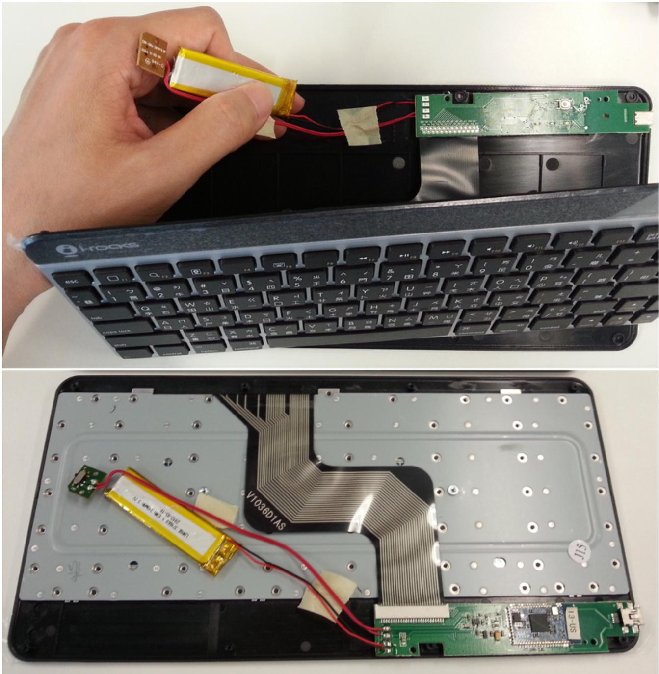
**Figure 8. Remove Battery From the Keyboard**
