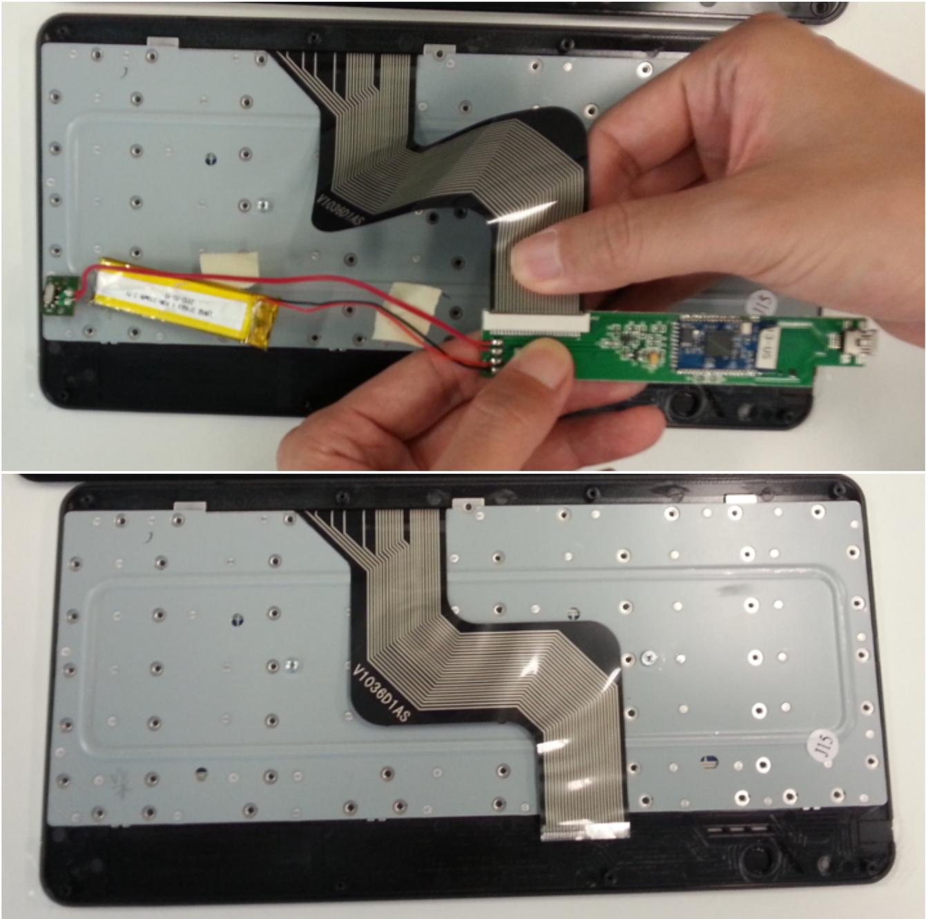
**Figure 9. Detach the 26-Pin FPC**
