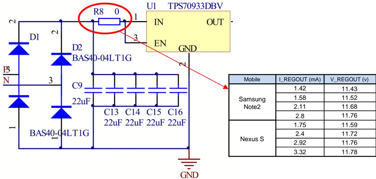
Figure 15. Power Received from NFC Antenna
