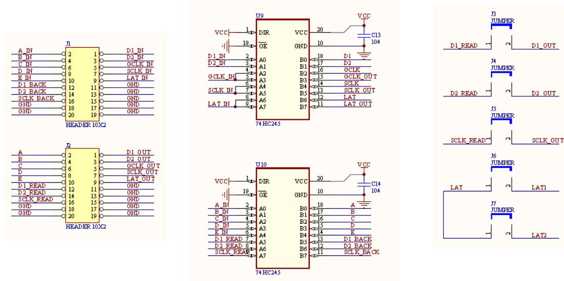
Line address decoder and protection circuit:
