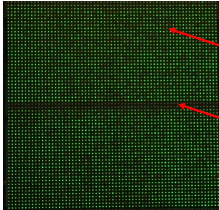
Below picture: GCLK=20.8MHz, LGSE function turn on to compensate blue/green LED.
