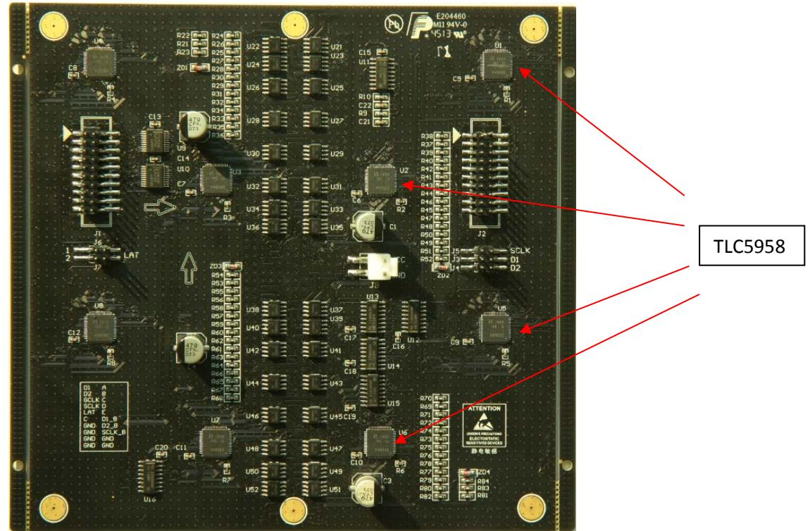
Fig2. Bottom view of LED module
