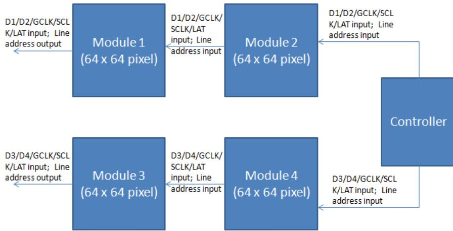
Module 1 and 2 are cascaded, use two GS data input ports D1 and D2. Same case for module 3 and 4. Because the total GS data transferred during one frame period is doubled, the minimum SCLK frequency should also be doubled.
