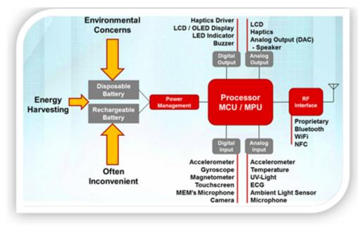
Figure 1. Simplified generic block diagram
