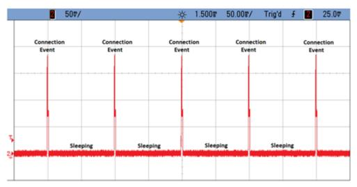
Figure 2. Typical RF energy usage profile
