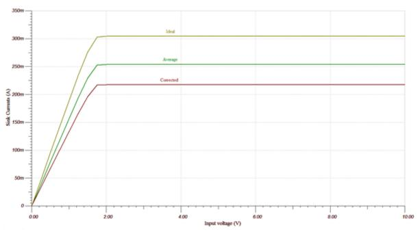
Figure 3. Sink Current vs. Drain Voltage for Ideal, Corrected, and Average R<sub>SETN</sub> Values
