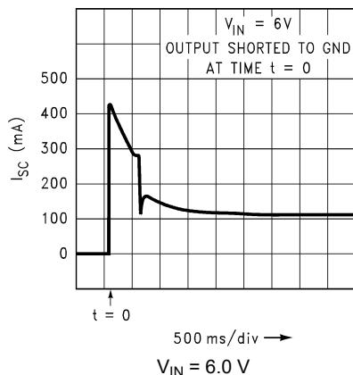
图 5-31. Short Circuit Current versus Time (Legacy Chip)
