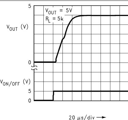
图 5-50. Turn-on Waveform (Legacy Chip)
