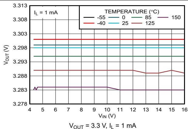
图 5-9. Output Voltage versus  $V_{IN}$  and Temperature (New Chip)
