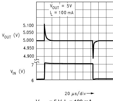
图 7-7. Line Transient Response (Legacy Chip)
