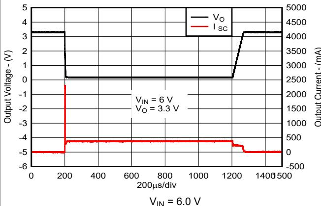
图 5-32. Short Circuit Current versus Time (New Chip)
