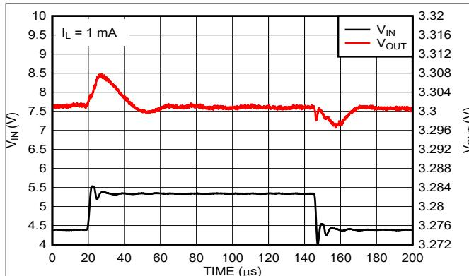
图 5-25. Line Transient Response (New Chip)
