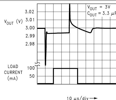
图 5-26. Load Transient Response (Legacy Chip)
