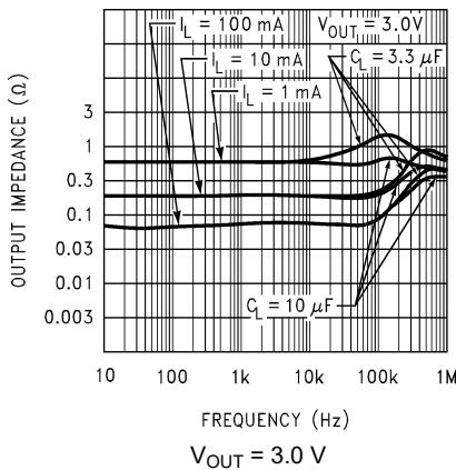
图 5-39. Output Impedance versus Frequency (Legacy Chip)
