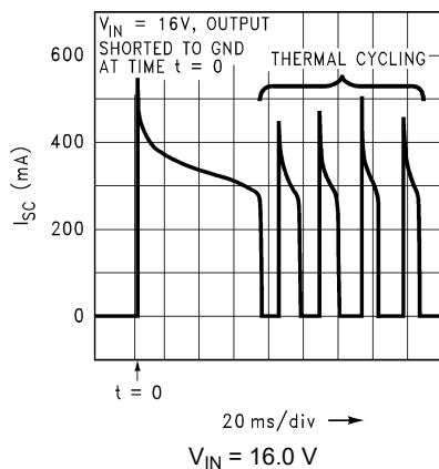
图 5-33. Short Circuit Current versus Time (Legacy Chip)
