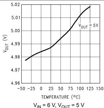
图 5-1. Output Voltage versus Temperature (Legacy Chip)
