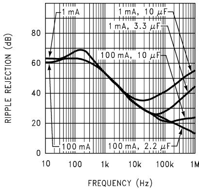
图 5-41. Ripple Rejection versus Frequency (Legacy Chip)
