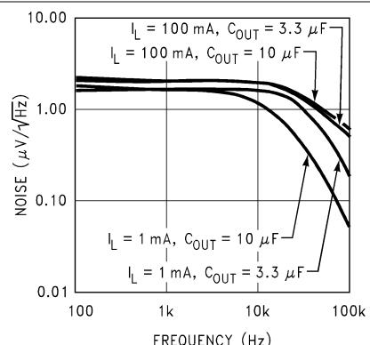
图 5-44. Output Noise Density versus Frequency (Legacy Chip)
