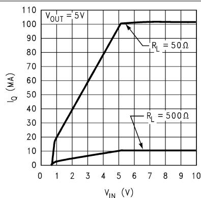
$V_{OUT} = 5 \text{ V}$ ,  $R_L = 500 \Omega$  and  $R_L = 50 \Omega$
