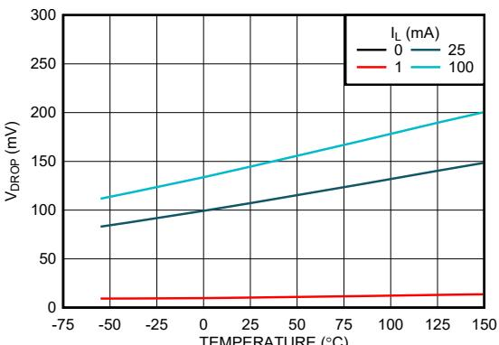
图 5-12. Dropout Voltage ( $V_{DO}$ ) versus Temperature (New Chip)
