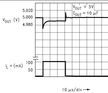
图 5-29. Load Transient Response (Legacy Chip)
