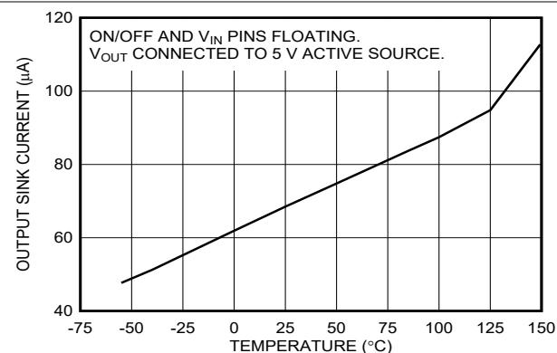
图 5-49. Output Reverse Leakage versus Temperature (New Chip)
