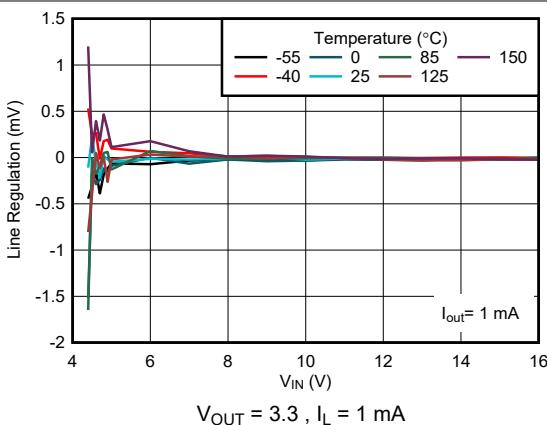
图 5-10. Line Regulation versus  $V_{IN}$  & Temperature (New Chip)
