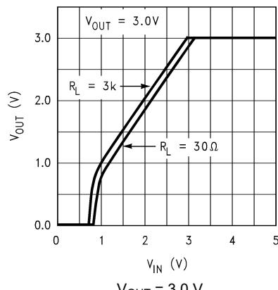
图 5-7. Output Voltage versus  $V_{IN}$  (Legacy Chip)
