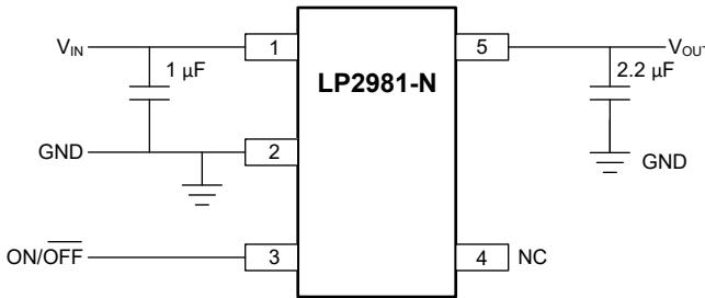
\*ON/ OFF input must be actively terminated. Tie to  $V_{IN}$  if this function is not to be used. Minimum output capacitance is shown to insure stability over full load current range. More capacitance provides superior dynamic performance and additional stability margin (see [#7.1.1](#)).
