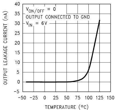
图 5-47. Input-to-Output Leakage versus Temperature (Legacy Chip)
