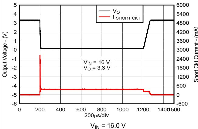
图 5-34. Short Circuit Current versus Time (New Chip)
