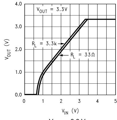
图 5-6. Output Voltage versus  $V_{IN}$  (Legacy Chip)
