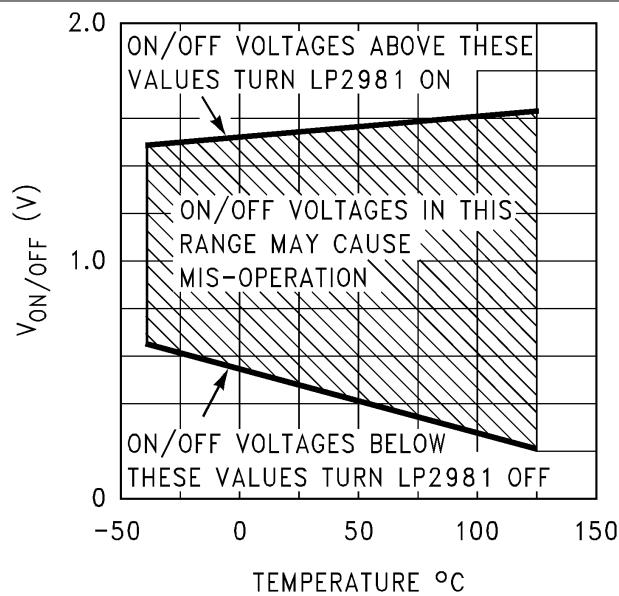
图 5-57. ON/ OFF Threshold versus Temperature (Legacy Chip)
