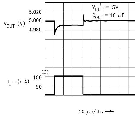
图 7-14. Load Transient Response (Legacy Chip)
