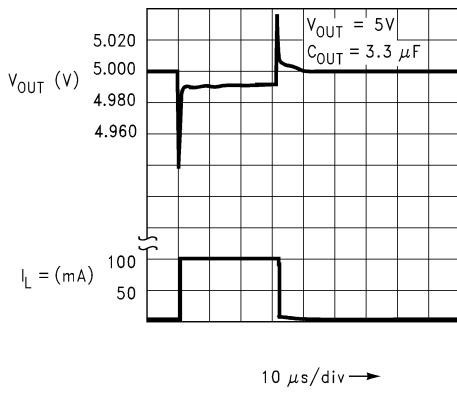
图 7-13. Load Transient Response (Legacy Chip)
