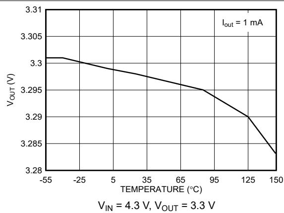
图 5-4. Output Voltage versus Temperature (New Chip)
