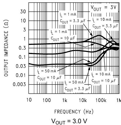
图 5-40. Output Impedance versus Frequency (Legacy Chip)
