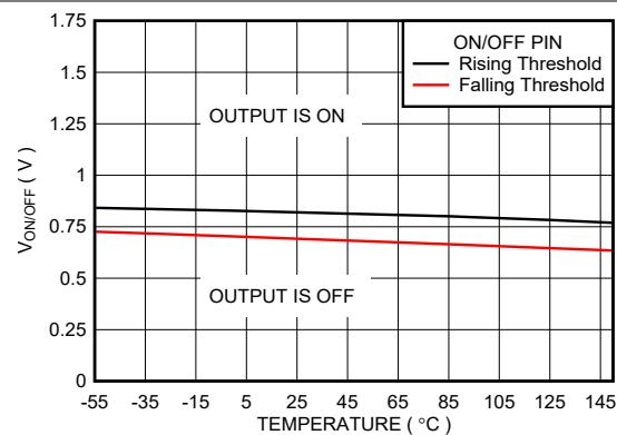
图 5-58. ON/ OFF Threshold versus Temperature (New Chip)
