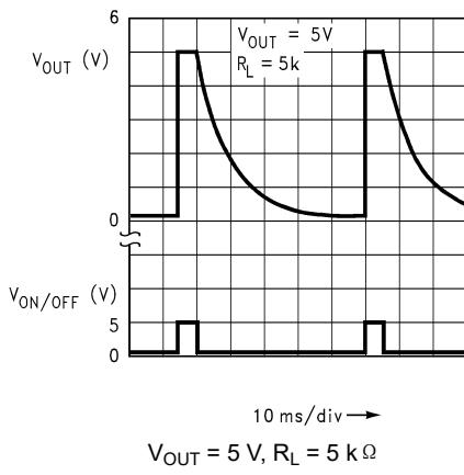
图 5-52. Turn-off Waveform (Legacy Chip)
