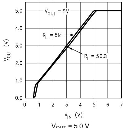
图 5-5. Output Voltage versus  $V_{IN}$  (Legacy Chip)
