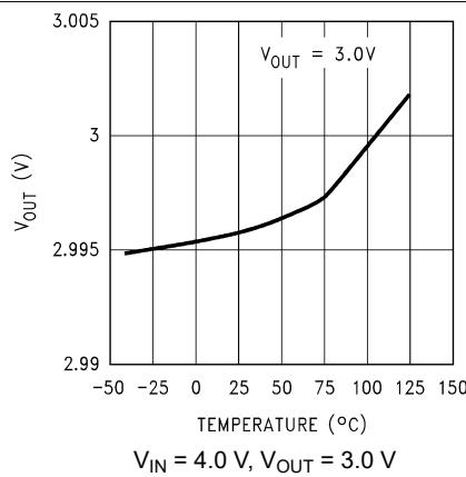
图 5-3. Output Voltage versus Temperature (Legacy Chip)
