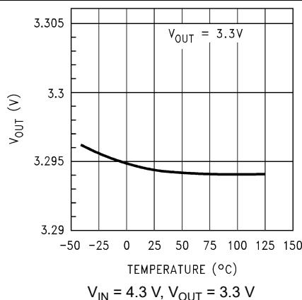
图 5-2. Output Voltage versus Temperature (Legacy Chip)
