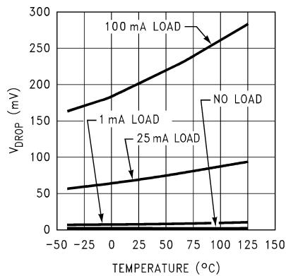
图 5-11. Dropout Voltage ( $V_{DO}$ ) versus Temperature (Legacy Chip)
