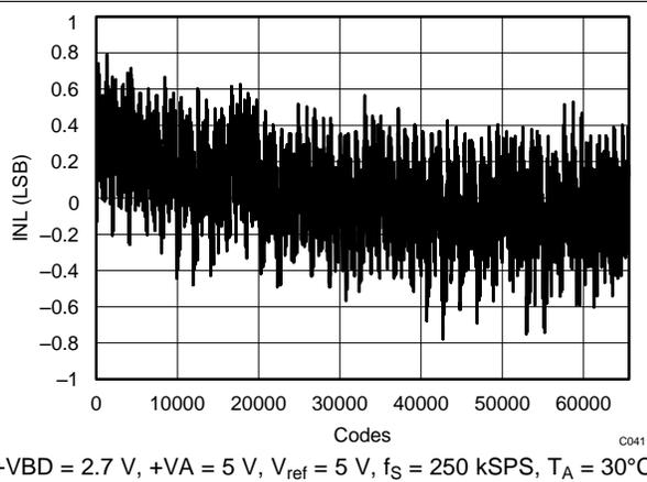
**Figure 41. INL Error vs Output Code**
