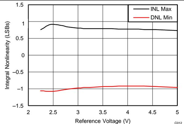
+VBD = 2.7 V, +VA = 5 V,  $f_S = 250\text{ kSPS}$ ,  $T_A = 30^\circ\text{C}$
