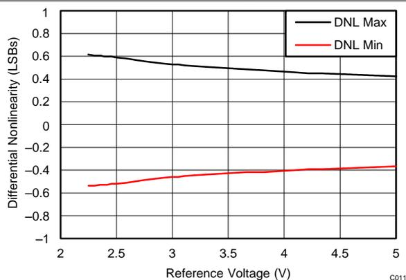
+VBD = 2.7 V, +VA = 5 V,  $f_S = 250\text{ kSPS}$ ,  $T_A = 30^\circ\text{C}$
