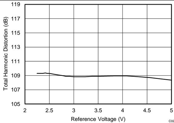
+VBD = 2.7 V, +VA = 5 V,  $f_{IN} = 1.9\text{ kHz}$ ,  $f_S = 250\text{ kSPS}$ ,  $T_A = 30^\circ\text{C}$
