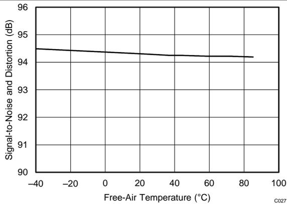
+VBD = 2.7 V, +VA = 5 V,  $V_{ref} = 5\text{ V}$ ,  $f_{IN} = 1.9\text{ kHz}$ ,  $f_S = 250\text{ kSPS}$
