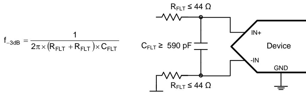
Figure 60. Antialiasing Filter
