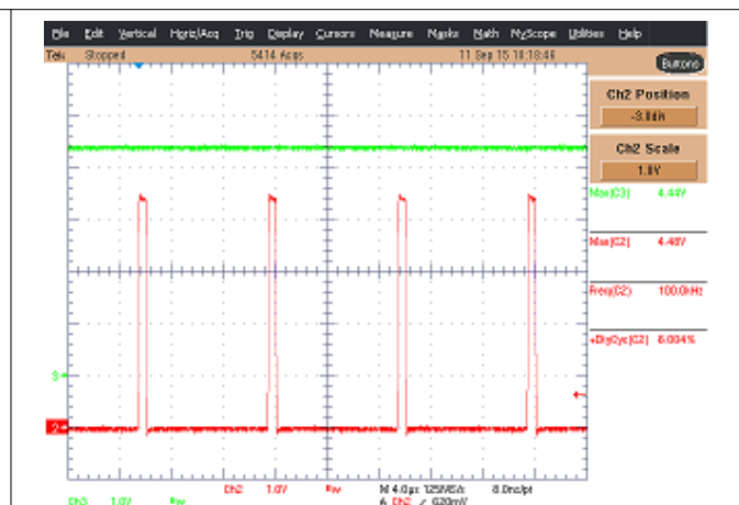
图 8-9. Supply Voltage 5 V Peak Signal 4.5 V
