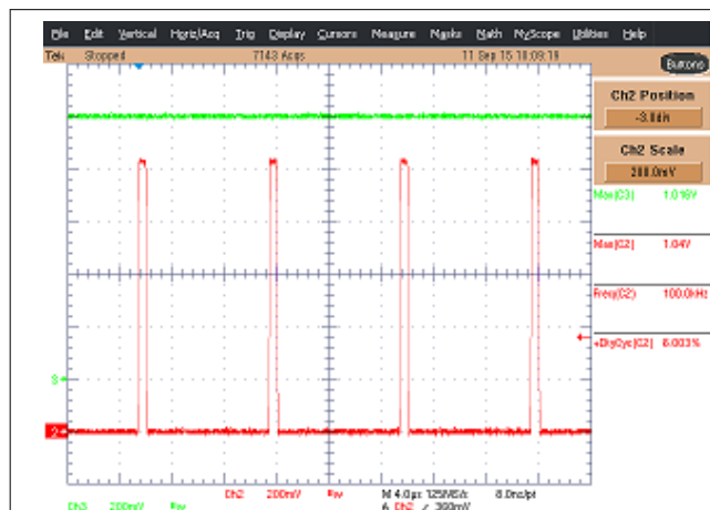
图 8-8. Supply Voltage 2.2 V, Peak Signal 1 V
