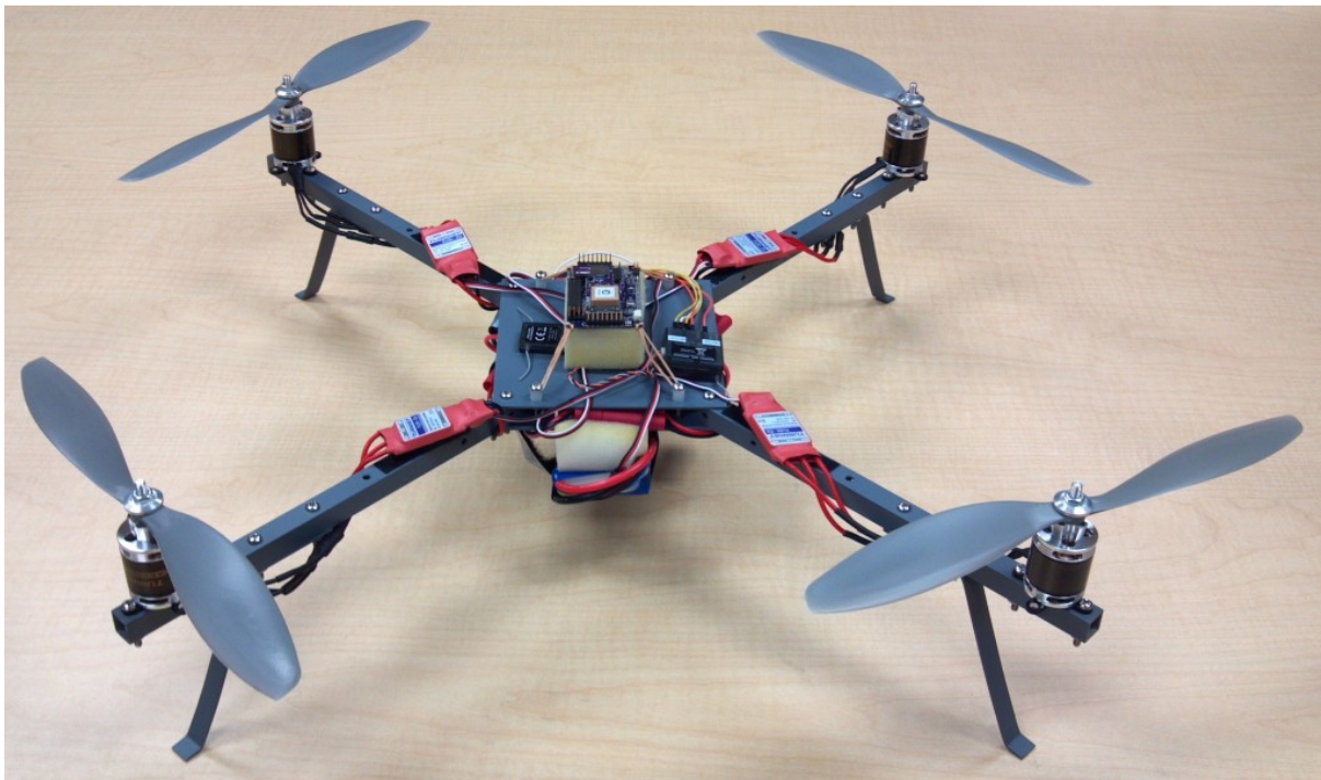
Figure 1. Research Drone with Commercial Motor Controllers Visible (SERL, 2014)
